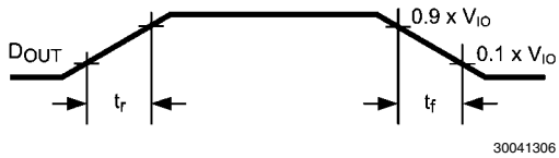
FIGURE 3. D_{OUT} Rise and Fall Times
